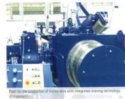
Plant for the production of trolley wire with coag and shaving technology. © Kieselstein
