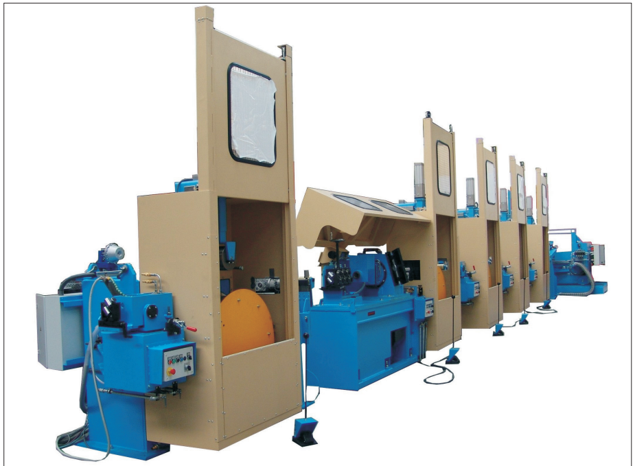
Trend to defect-free surface qualities requires the systems continuous enhancement: draw-peeling line. Photos: Kieselstein
