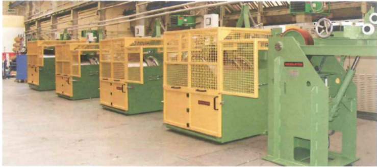
Drawing plant for the production of trolley wire.
