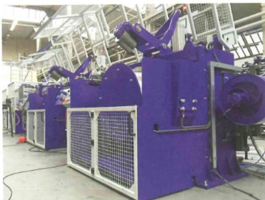
Plant for drawing and shaving of casted wire.
