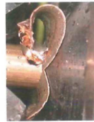
Chip removal by shaving.
