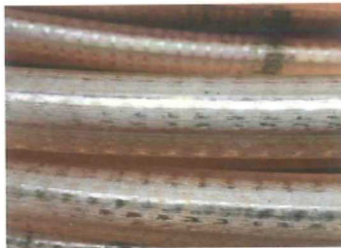
Detail casted wire, here copper-magnesium-alloy. Photos: Kieselstein
