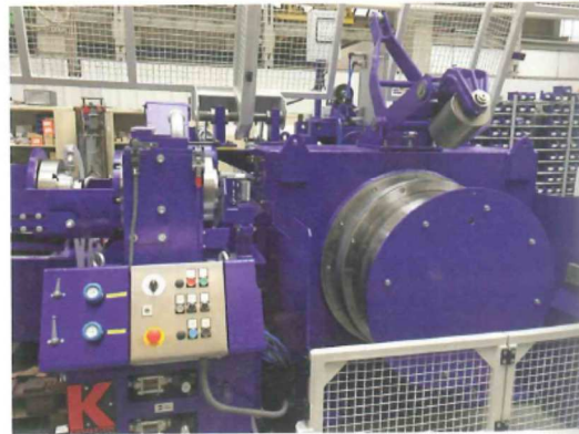
Drawing block with integrated shaving unit.
