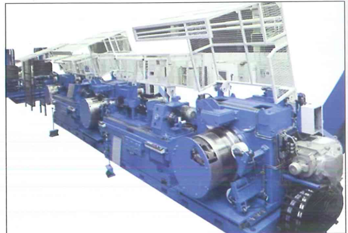
Picture 8: Drawing and draw-peeling plant [source KIESELSTEIN]
