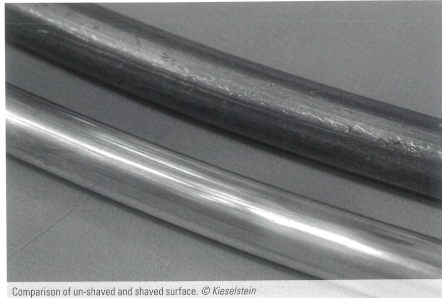
Comparison of un-shaved and shaved surface. © Kieselstein
